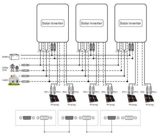
3. Four parallel-connected solar storage inverters:
