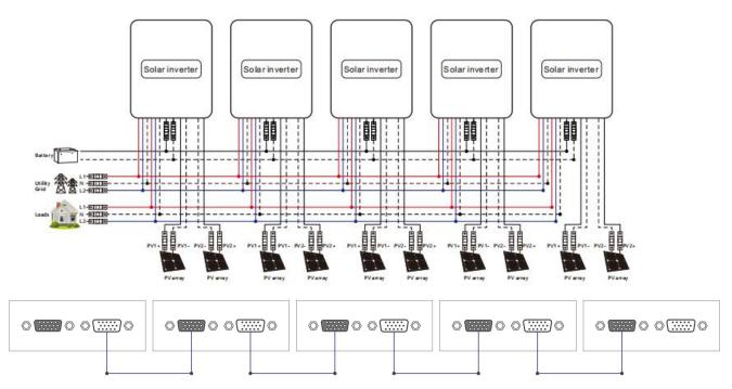
e. Six parallel-connected solar storage inverters:
