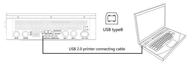
Users can use the upper computer software through the port to read and modify device parameters. If needing the installation package for the upper computer software, you can download it from the official website of SRNE, or contact us to get it.
