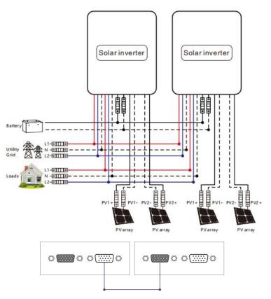
b. Three parallel-connected solar storage inverters:
